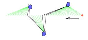
Fig. 9. Example of implicit coordination. Green (bright) lines represent that only one robot would approach the ball at this position. Black lines show when coordination is predicted to likely fail. The robots must all approach the ball from the right.
